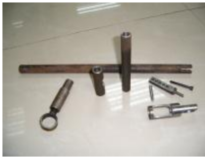
SST for valve oil seal
